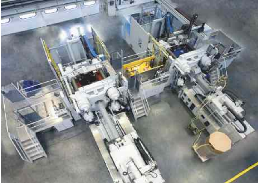
1300 ton Engel IMM with 15 ton moulds Mould change time is 47 seconds
